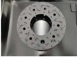
Fig. 3. Assembly of getters developed.
